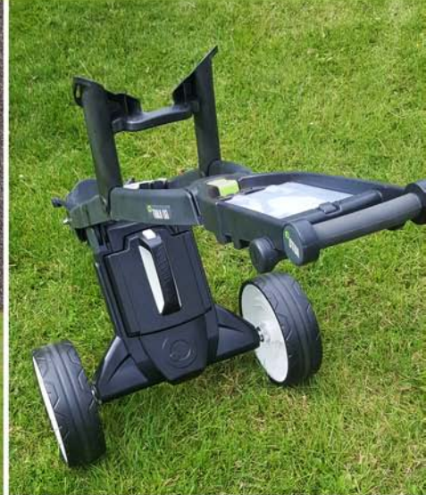
T1 mouldings of the battery housing assembled to the original GoKart trolley arms.
