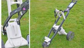
The trolley was modified to accommodate the new mouldings developed using CAD & sketch models.
